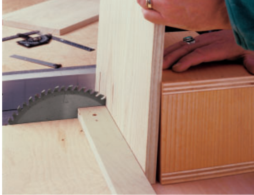
Photo F: A simple table-saw jig positions the workpiece to cut the angled cheeks of the tenons.
