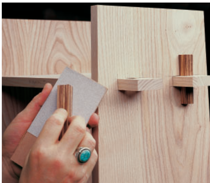
Photo J: Sand the tapered faces of the wedges until they all sit at the same height.
